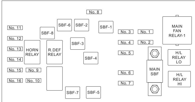
SECONDARY AIR FUSE &amp; RELAY BOX
